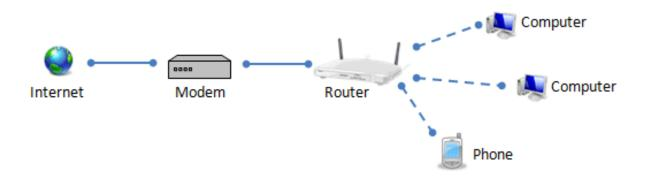
All the devices that are connected to your router forms a network. This is what allows your devices to "talk" to each other – for example, if you have a Wi-Fi printer, you can print wirelessly if the device you're printing from and your printer are all on the same network.
